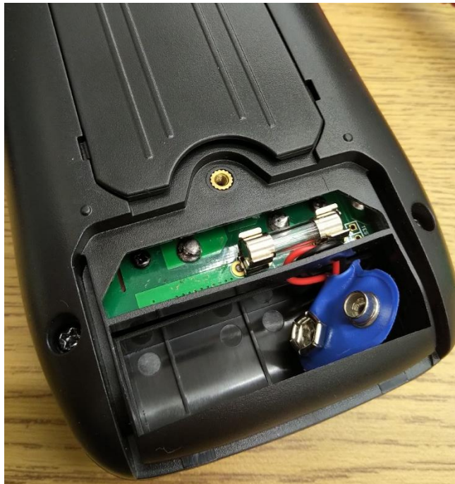
Figure 11: Removed battery and exposed fuse
